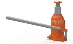
A complete range of hydraulic bottle jacks for any kind of lifting. Solid, strong structure, and a wide support base, guarantee stability in all the correct operating positions. Equipped with an adjustable extension screw with safety stop, the jack are also furnished with an automatic end stroke safety valve.
