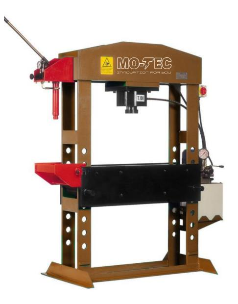
New series of motor driven three-phase press (230.400V) with automatic double speed gearbox. Supplied with an extra side piston, 12 ton capacity, with manual pump. Complete of gauges, "v" blocks and plate. Hoisting of working table by chains. The presses are supplied with oil and plate for protection of the rod. The machines are designed and manufactured as per the last CE directives. Thanks to the system "Safety Off" it is possible to adjust the machine safely and easily.
