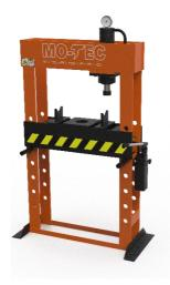
Two speed hand pump hydraulic presses with automatic re-entry of the piston. By closing the two upper hand wheels on gets the fast piston approach. By opening the side upper hand wheels on gets the high pressure. All the presses are supplied with two "v" blocks, plate and gauge to control the working pressure.
