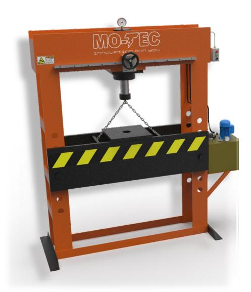
New series of automatic double speed motor driven press with mobile ram, complete of gauge and double automatic speed gearbox with three phase motor (230-400V). thanks to his gears pump it is possible to have a quick approach and return of the piston, while for the working phase it has a radial piston pump to get the high pressure. Thanks to the adjustable ram device, it is possible to make different operations on one piece when the remotion of the same result too difficult and expensive.
