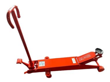
Hydraulic trolley jacks for lifting stated capacity loads. Solid and strong structure fitted with four wheels; two fixed and two swivel, guarantees stability in all the correct operating position. All the models are supplied with pedal for quick approach of the loads, removable handle for quick and easy transport. Equipped with automatic end stroke safety valve and overload valve. On request all t models till 5 ton capacity can be supplied with nylon and or wulkolan wheels.
