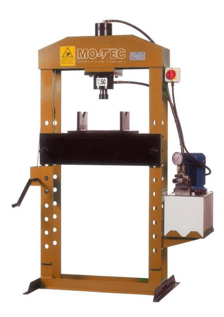
Hydraulic presses with three phase motor driven (230-4000 v.) with hydraulic gearbox. All the presses have a calibration valve, and a three-position drive distributor (feed-neutral-return). All the machines are supplied with two "V" blocks, plate and gauge to control the working pressure. The hoisting of the working table is manual for the 10 and 20 ton, while the other model are supplied with a manual whinch.
